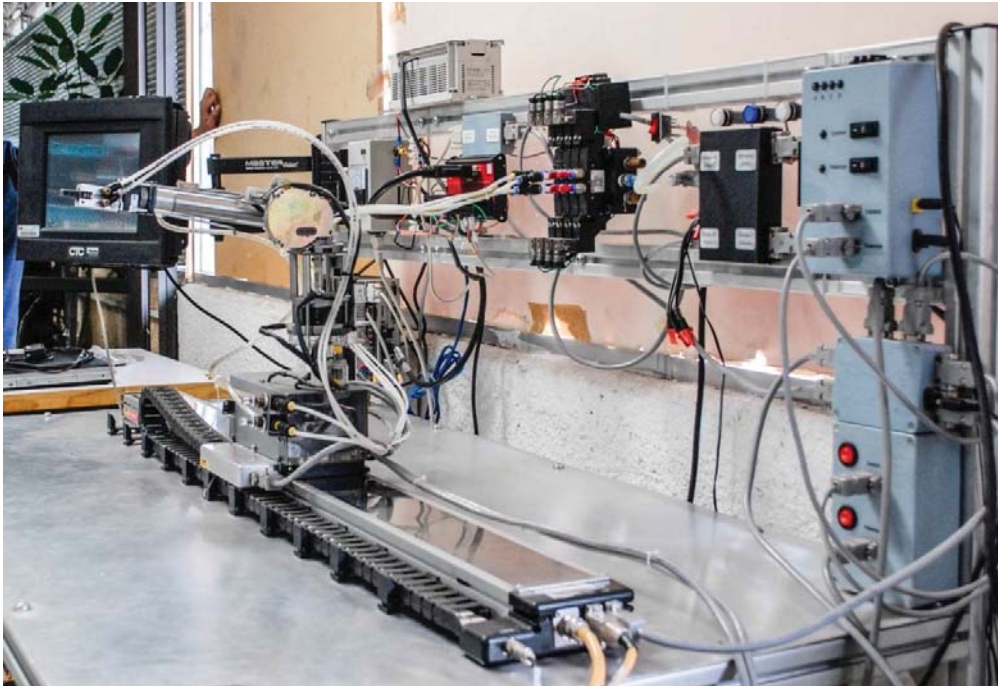
Figure 1. Actuators arranged on a spherical coordinates system, over the servomotor platform.
