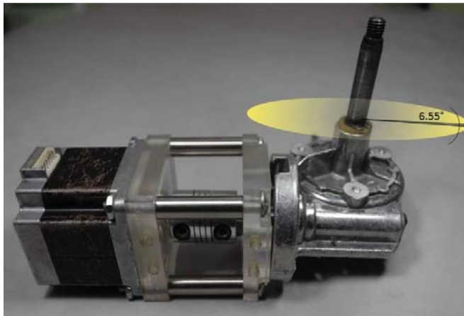
Figure 2. The crown's angular advance is 6.55^\circ for each revolution in the stepper motor.
