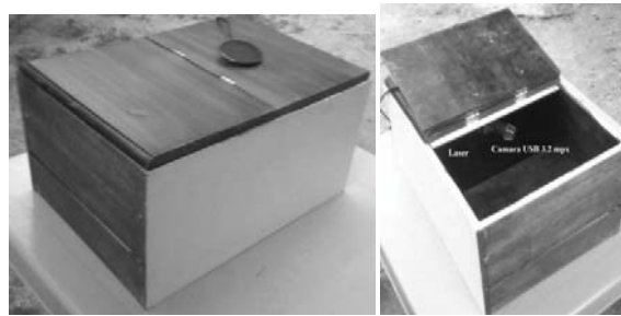
Figure 5. Prototype for capturing images of objects of study
