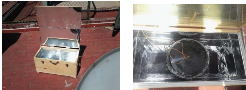
Figure 1 Solar cooker box-type: with exterior reflectors and interior reflectors
