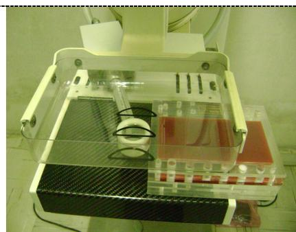
**Figure 1.** Ionization chamber positioned adjacent to and in the same plane of the phantom of 5 cm height and centralized along with "Bucky" of mammography equipment.
