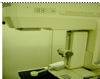
**Figure 2.** Ionization chamber positioned in the center of the field of radiation (FCC= 59 cm) for the  $Ka,i$  measurements.
