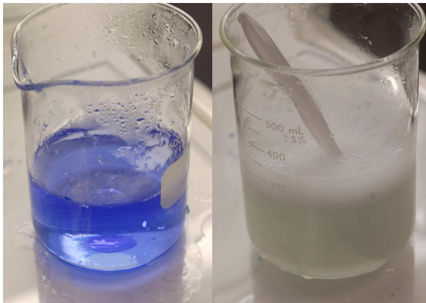
Figure 1. Oxidative decomposition of leuco-crystal violet hydrogel dosimeter: left panel, before treatment, right panel, sample after two hour reaction with bicarbonate and hydrogen peroxide.
