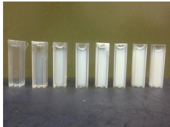
Figure 3. Irradiated PAGAT gel
