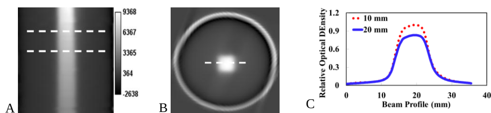
Figure 3. A. Central slice of reconstructed dosimeter image; B. Axial slice at the depth of 20mm; C. Beam profiles along central cross lines of the field at depths of 10 and 20mm.
