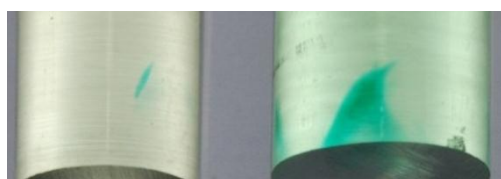
Figure 2. Colour changes observed when PRESAGE® was exposed to 7.87 MPa peak negative pressure HIFU. The left sample is a ‘soft’ one made of CF95 polyurethane and the right is the “hard” SO206 polyurethane.
