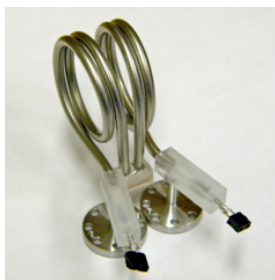
Figure 3. Multi-turn and gradiometric sensing arm for a SHeQUID. The length of the arm is approximately 0.5m. From Ref [28].
