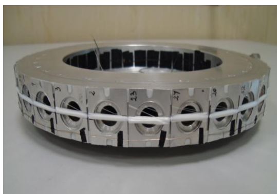
Figure 1. The circular holder and attached to it plates with the PET filaments.
