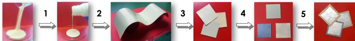
Figure 1. Fabrication process of investigated samples: 1. Preparation of a pourable slurry from PZT, organic and sintering additives, 2. Tape casting of films, 3. Punching out green bodies, 4. Debinding and sintering, 5. Metallizing with Ag varnish and poling with 3 kV/mm.
