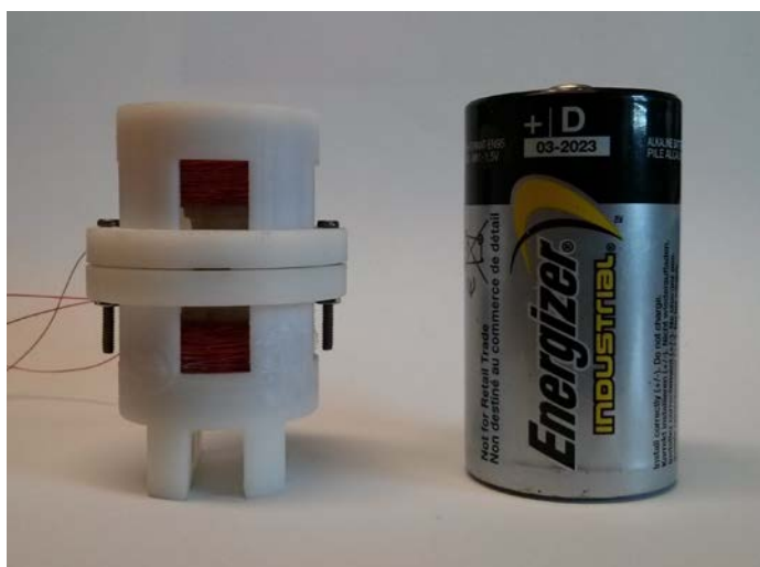
(a) Assembled energy harvester
