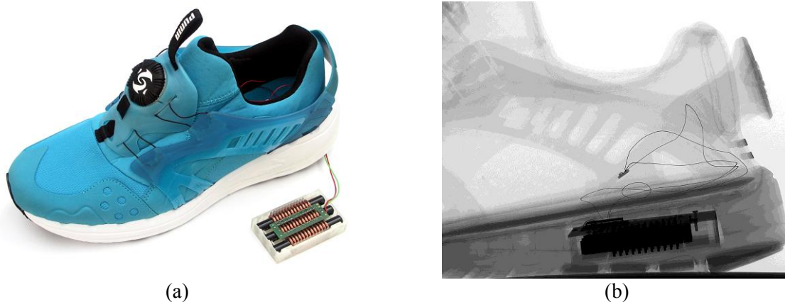
Figure 4. (a) Sports shoe with integrated harvester and a second device by its side. (b) X-ray photography of the shoe showing the harvester system. The temperature sensor and the wireless data transmission chip from the sample application can be seen.
