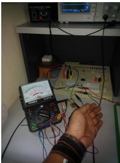
Figure 4. A pilot test of the transducer system was performed on the subject left hand. An oscilloscope and a multimeter were used to observe the evoked potentials. The instrument used were Tetronix TBS 1062 oscilloscope and Tenma 72-8170 multimeter.
