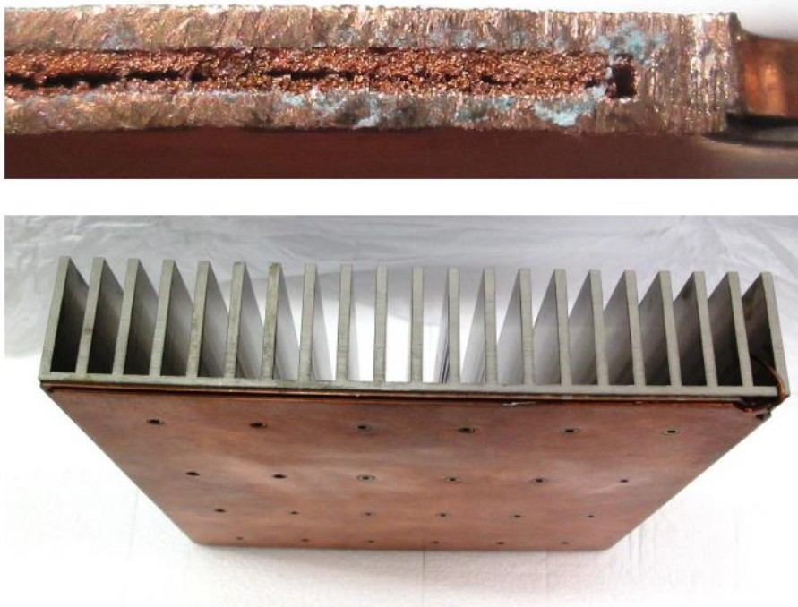
Figure 3. Image of the VCHS cross section and overall composition.
