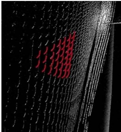
Figure 12. A part of a point cloud of a 3D scan, a few profiles are highlighted in red
