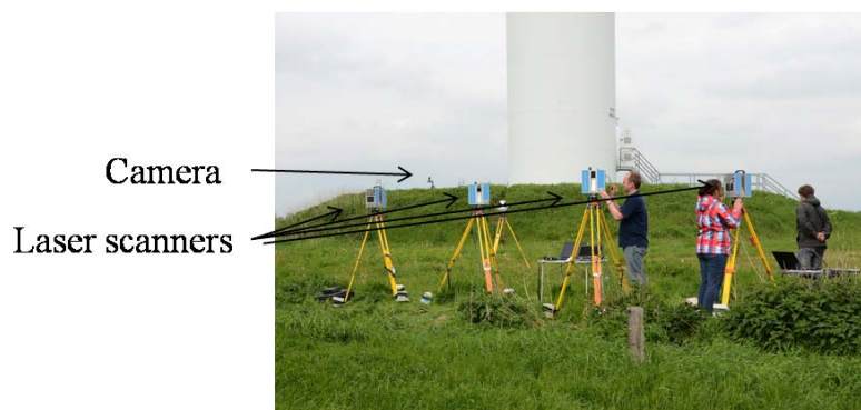
Figure 4. Camera and four laser scanners in the field
