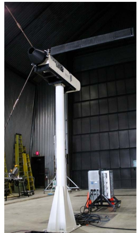
Figure 6. Assembled test rig and rotor
