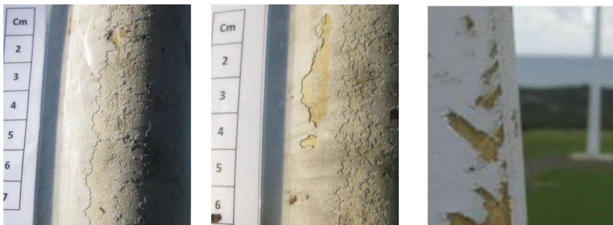
Figure 1. Examples of LE erosion.
