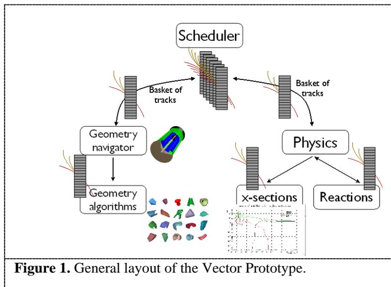
**Figure 1.** General layout of the Vector Prototype.
