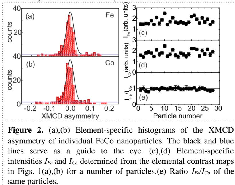
**Figure 2.** (a),(b) Element-specific histograms of the XMCD asymmetry of individual FeCo nanoparticles. The black and blue lines serve as a guide to the eye. (c),(d) Element-specific intensities  $I_{Fe}$  and  $I_{Co}$  determined from the elemental contrast maps in Figs. 1(a),(b) for a number of particles.(e) Ratio  $I_{Fe}/I_{Co}$  of the same particles.
