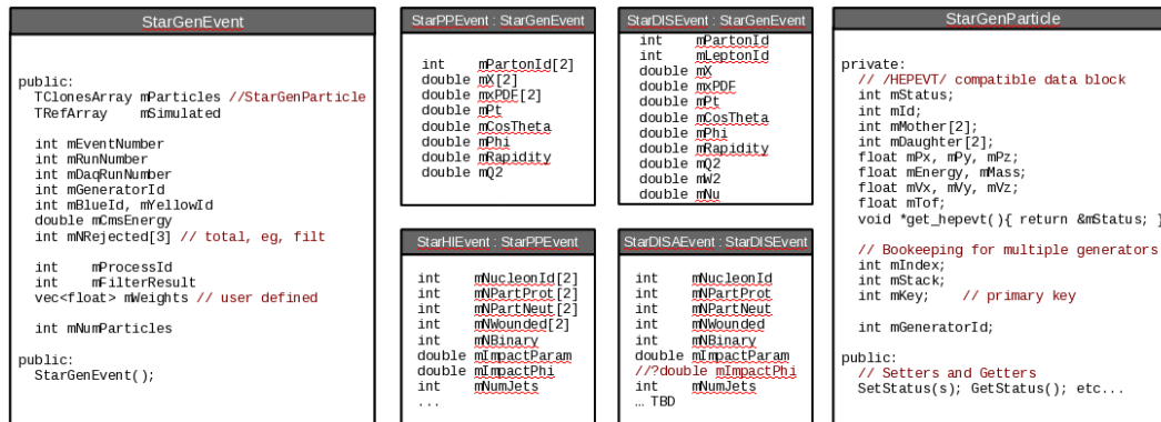
Figure 1. The StarGenEvent event record provides persistency for common header information and particles. Derived classes represent the different kinematics of pp , pA , AA , ep and eA collisions. A lightweight particle class is also provided, extending the HEPEVT standard with additional bookkeeping values which enable us to trace the particle back to the parent generator.
