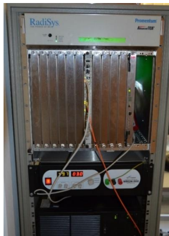
Figure 2. Test setup with a RadiSys Promontum ATCA Sys-6010 crate with Dual Star backplane instrumented with a FPGA test board (right most board), a 10 GbE RadiSys ATCA-2210 switch blade (centered board) and a dual Intel Xeon QuadCore based PC with four dual-port 10 GbE Myricom 8B2-2S (bottom) network interface cards.
