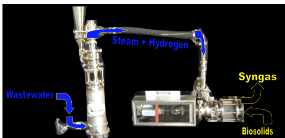
Figure 1. Plasma gasification of sewage and solid waste using a dual plasma system (Courtesy of Foret Plasma Labs).
