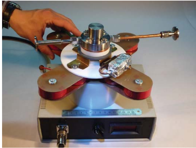
Figure 1. PF-2J: a portable plasma focus device.
