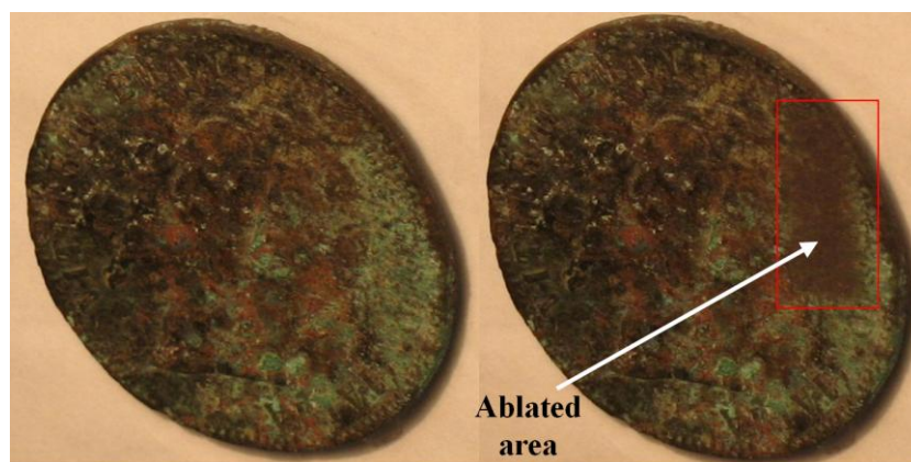
Figure 5. Photo of a virgin (left) and a processed coin (right).
