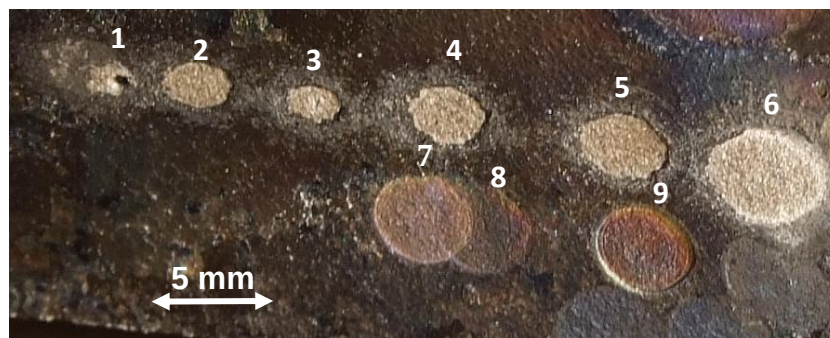
Figure 7. Macro-photography of a part of the investigated deuterized-graphite target, which shows micro-craters formed after the irradiation at different focusing length ( f = 50 \text{ cm} and 70 \text{ cm} ) and different distances of the lenses from the target ( l_f = 70 \text{ cm} , 75 \text{ cm} and 80 \text{ cm} ). All craters were produced by the 1063\text{-nm} laser pulses. The crater no. 1 was produced at f = 70 \text{ cm} and l_f = 75 \text{ cm} ; the crater no. 2 was produced by at f = 70 \text{ cm} and l_f = 80 \text{ cm} ; the crater no. 3 - at f = 70 \text{ cm} and l_f = 85 \text{ cm} ; the craters nos. 4 and 5 - at f = 70 \text{ cm} and l_f = 70 \text{ cm} ; the crater no. 6 - at f = 50 \text{ cm} and l_f = 70 \text{ cm} ; the crater no. 7 - at f = 50 \text{ cm} and l_f = 80 \text{ cm} ; and craters nos. 8 and 9 were produced at f = 50 \text{ cm} and l_f = 75 \text{ cm} .
