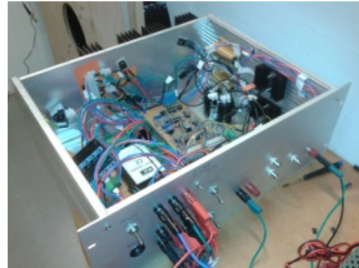
Figure 2. Photograph of the amplifier enclosure with the top plate removed.
