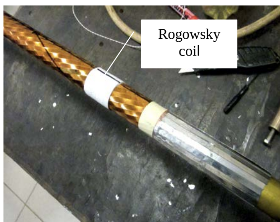
Figure 1. First layer of a cable core model with Rogovsky coil installed.
