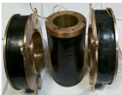
Figure 3. Superconducting magnet (disassembled).
