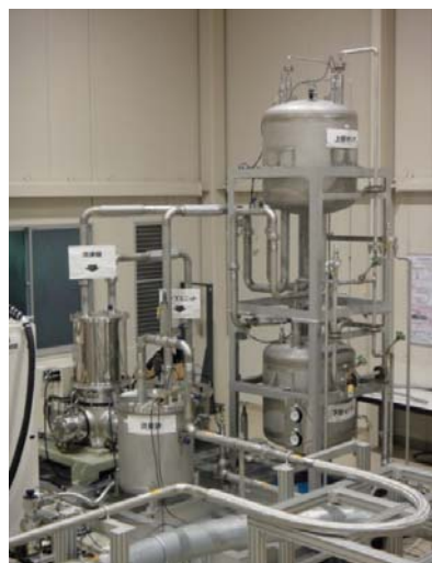
Figure 2. Cryogenic system in CASER-2
