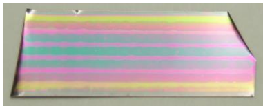
Figure 2. Photograph of inkjet printed \text{CeO}_2 filaments on a RABiTS substrate.
