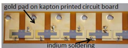
Figure 4. Resistors soldered on kapton-gold strip
