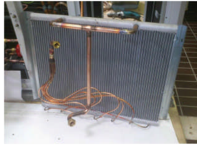
Figure 3. A picture of the mini-channel heat exchanger.
