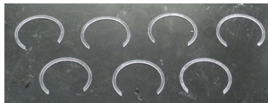
(c) Spacer; PMMA ring 0.5~4 mm
