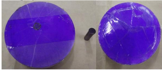
Figure 6. Deformation and fracture modes of H-B projectile and target at velocity 161.3 m/s.
