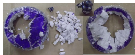
Figure 13. Deformation and fracture modes S-B projectile and target at velocity 801.1 m/s.
