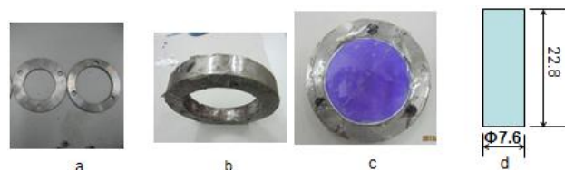
Figure 2. Target system and projectile. (a) cover ring; (b) hoop outside the ceramic target; (c) ceramic target (d) projectile shape and size.
