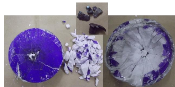
Figure 11. Deformation and fracture modes S-B projectile and target at velocity 610.3 m/s.
