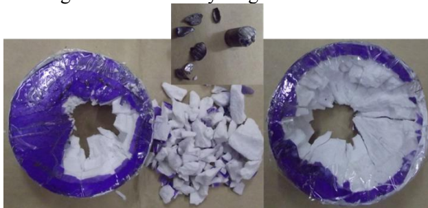
Figure 10. Deformation and fracture modes H-B projectile and target at velocity 610.3 m/s.
