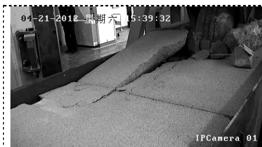
Figure 3. Foamed concrete in front of the wheel
