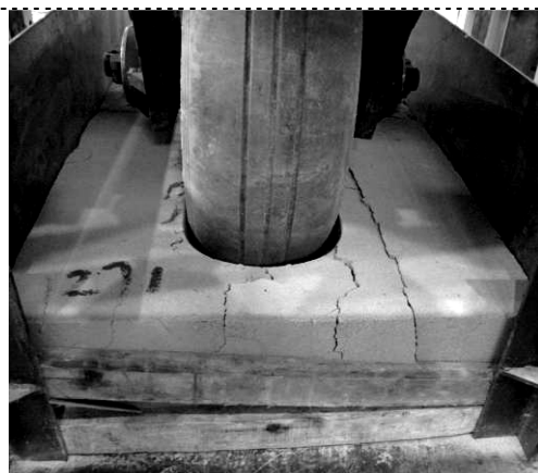
Figure 3. Foamed concrete in front of the wheel
