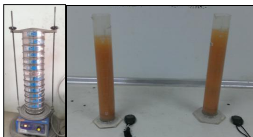
Figure 4. Mechanical sieve (left) and hydrometer test (right).
