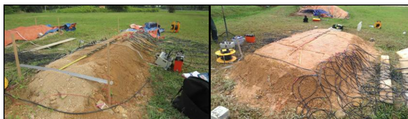
Figure 1. Soil model (lateritic soil) tested by 2D electrical resistivity test: Loose condition (left) and dense condition (right).
