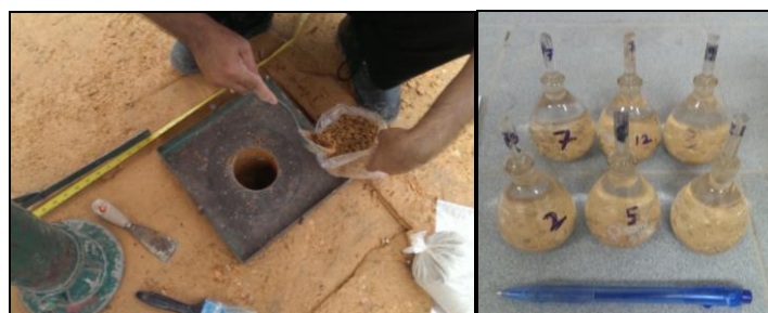
Figure 3. Field density test (left) and specific gravity test (right).
