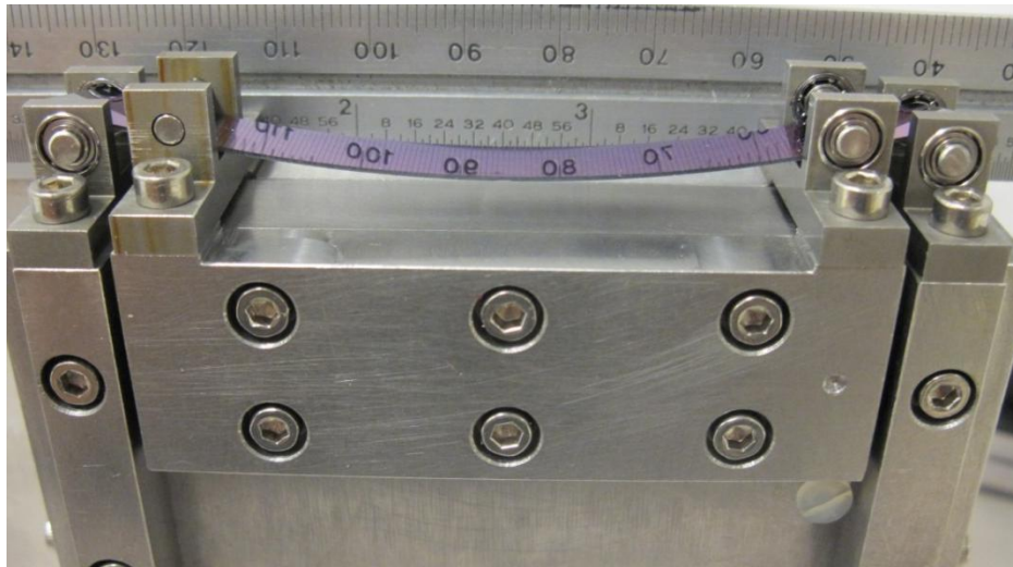
Figure 2: “Bar analyzer” bent in a simple bending apparatus. The diffraction plane contains the bend axis and is normal to crystal surface. Bending occurs when the pair of inner rods move down relative to outer rods. All 4 rods are free to rotate.
