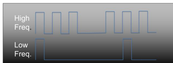
Figure 3. High and low frequency outputs from V2F.
