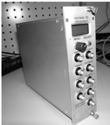
Figure 2. APS Voltage to Frequency Converter.
