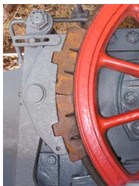
Figure 6. Unit test. One wheel. One brake. Stopping power can be measured.
