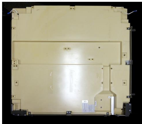
Figure 1. EPID viewed from underneath showing the indentation in the rear housing
