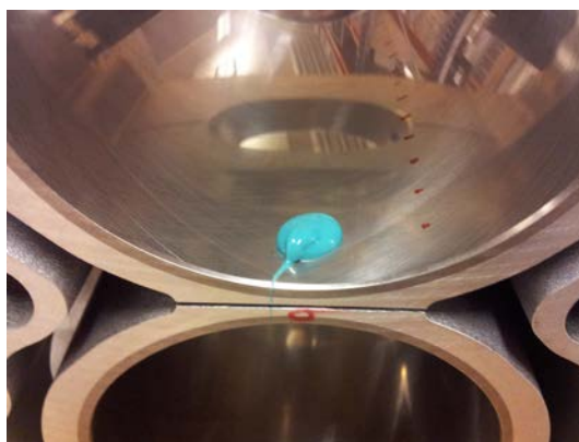
Figure 4. Replication of liner surfaces for different depth in order to measure with the interferometer.
