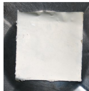
Figure 2 (b). Picture of the palladium membrane after the selective etching of copper foil for the back side, resulting in a free standing & mechanically stable palladium membrane.
