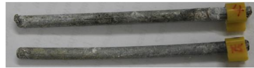
Figure 2. Non-nitrated sample (top) Nitrated sample (bottom).
