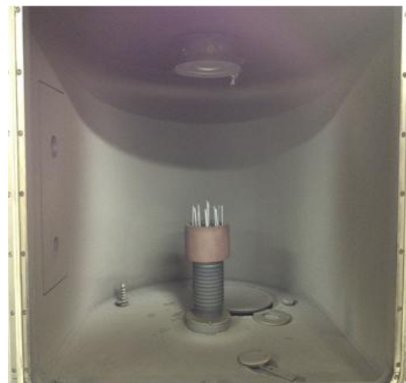
Figure 4. 3DII Implantation process.
