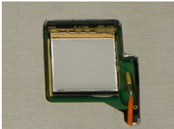
Figure 1. InGrid mounted in the anode of the detector.
