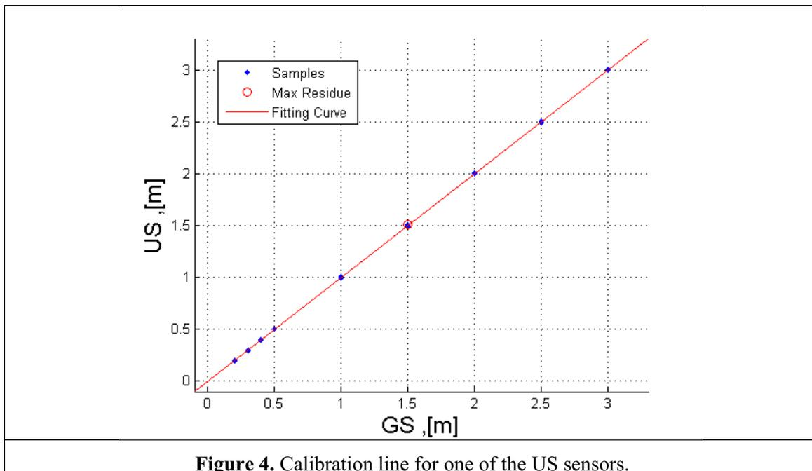
**Figure 4.** Calibration line for one of the US sensors.
