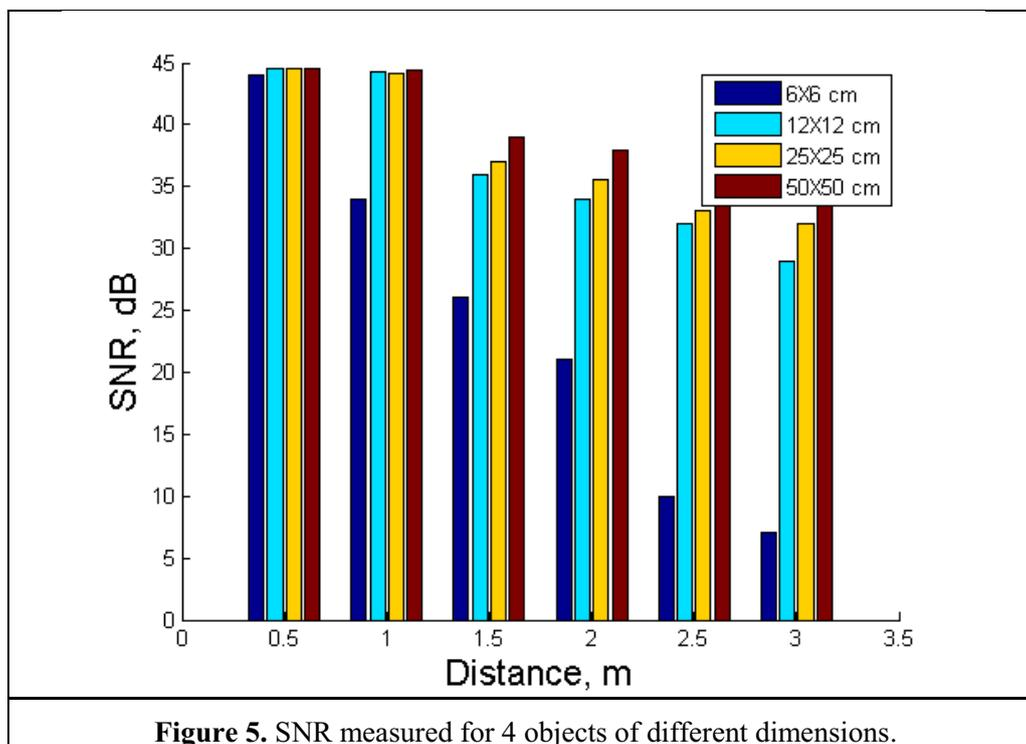
**Figure 5.** SNR measured for 4 objects of different dimensions.
