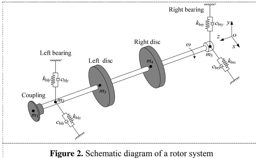
**Figure 2.** Schematic diagram of a rotor system
