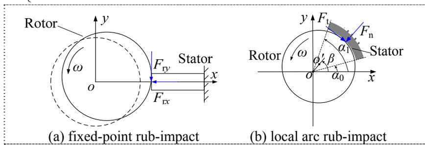
**Figure 1.** Schematic diagrams of fixed-point and local arc rub-impacts
