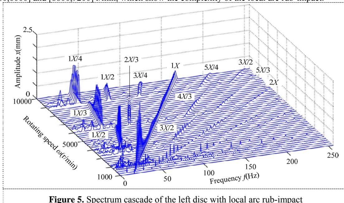
**Figure 5.** Spectrum cascade of the left disc with local arc rub-impact
