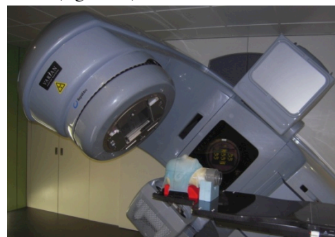
Figure 4: Irradiation treatment of the gel dosimeter head phantom
