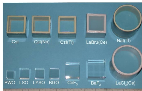
Figure 2. Comparison of different cubic scintillator materials shown with dimensions of 1.5X_0 . The picture is taken from [8].
