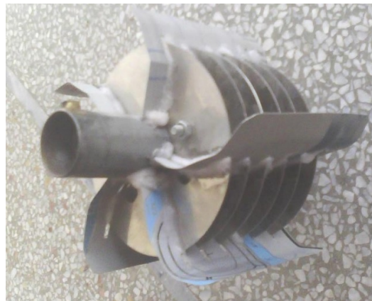
Figure 4. Rotor of the physically made prototype new design tesla turbine.
